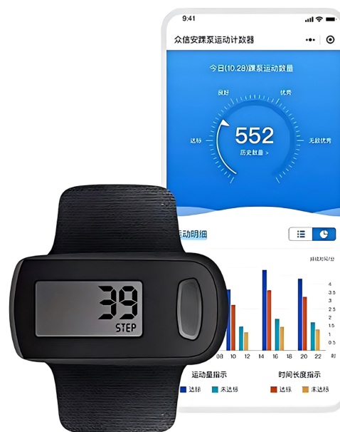
Fig. 4. The appearance of the telemonitored APE and the display of the software on the mobile phone.
