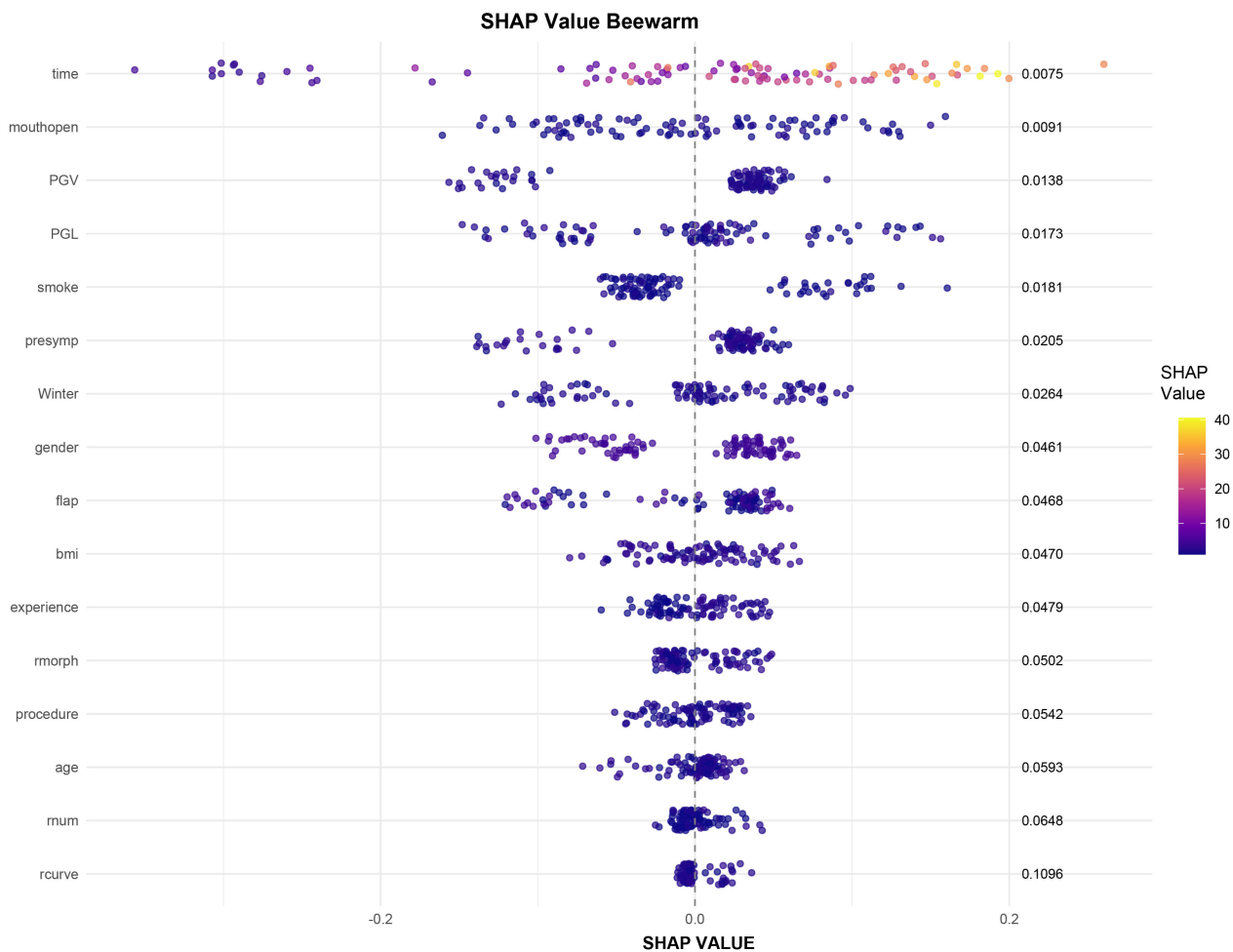
Fig. 2. SHapley Additive exPlanations (SHAP) values in a beeswarm plot for GBM. SHAP values in a beeswarm plot summarize the contribution of each feature to the model's predictions. Each point on the plot represents the SHAP value of a single observation for a particular feature. The x-axis represents the SHAP value, which quantifies the impact of the feature on the model output. A positive SHAP value indicates that the feature value for that observation increased the prediction, while a negative SHAP value indicates that it decreased the prediction. The features are ranked in descending order of their overall importance, determined by the average absolute SHAP value across all observations (represented by the values on the y-axis to the right of each feature's beeswarm). PGV, Pell-Gregory vertical; PGL, Pell-Gregory level.
